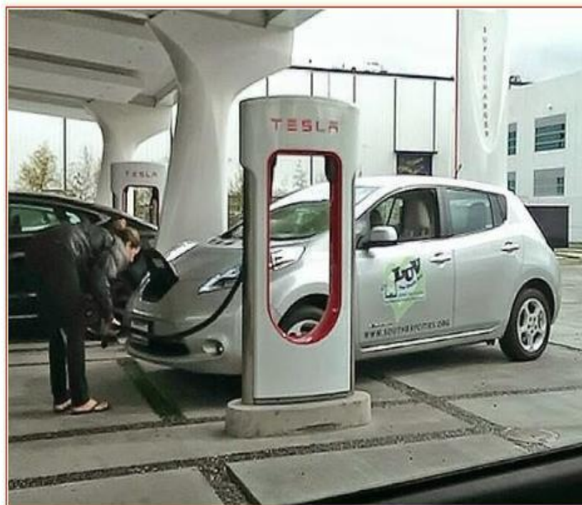
SuperCharger cord doesn't fit the CHAdeMO socket
