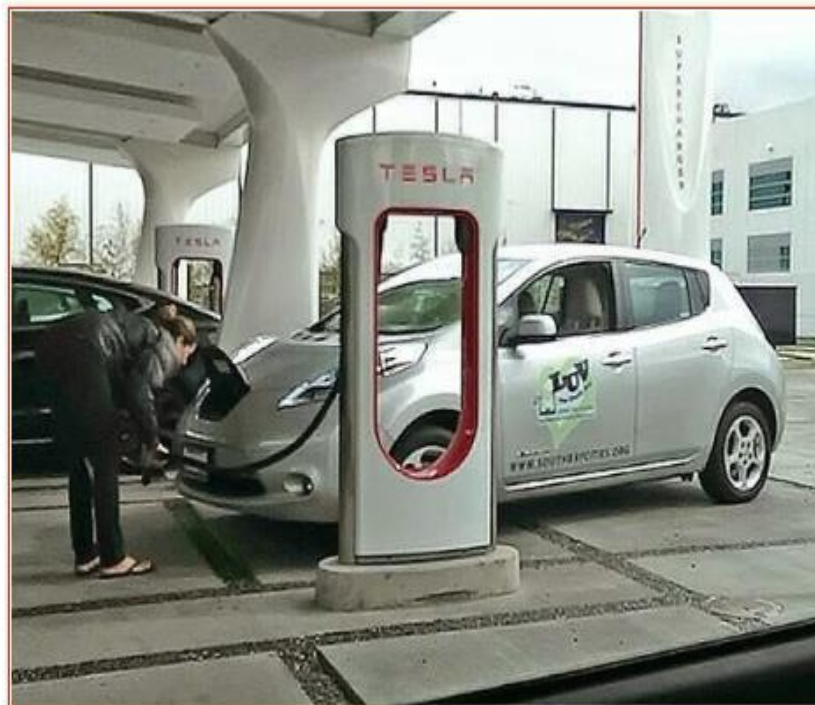
SuperCharger cord doesn't fit the CHAdeMO socket
