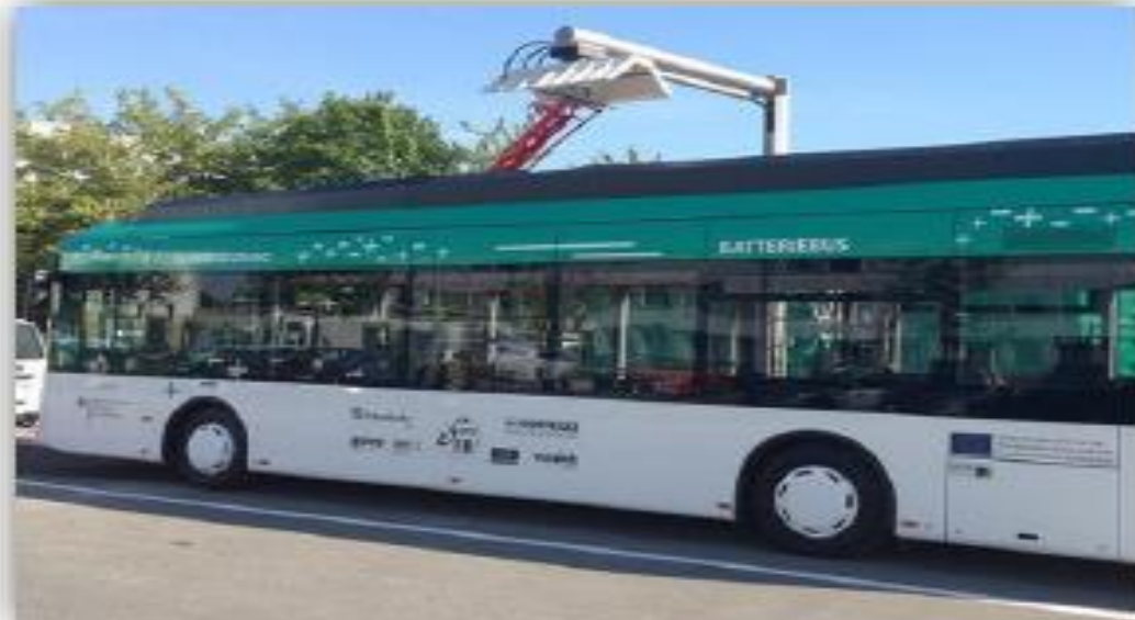
Automatic Connection Device (ACD) Pantograph (Up or Down)
